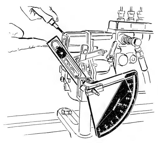
Drive injection-pump assembly at prescribed speed. Move control lever in direction of full load until prescribed control-rod travel has been attained. Read off position of control lever from adjusting tool 0 681 440 006 or 1 688 130 183 and compare to maximum value specified in test-specification sheet.
